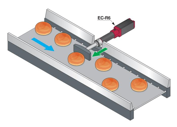
**Explanation** A simple, inexpensive Elecylinder is used here for the application was between the two points.
