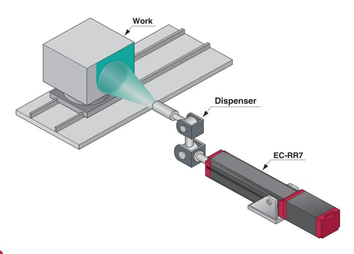
Explanation The angle of the spray gun can be adjusted by converting linear motion of the rod type Elecylinder into oscillating motion. The spray gun speed and movable range can be easily changed, making coating work easier.
