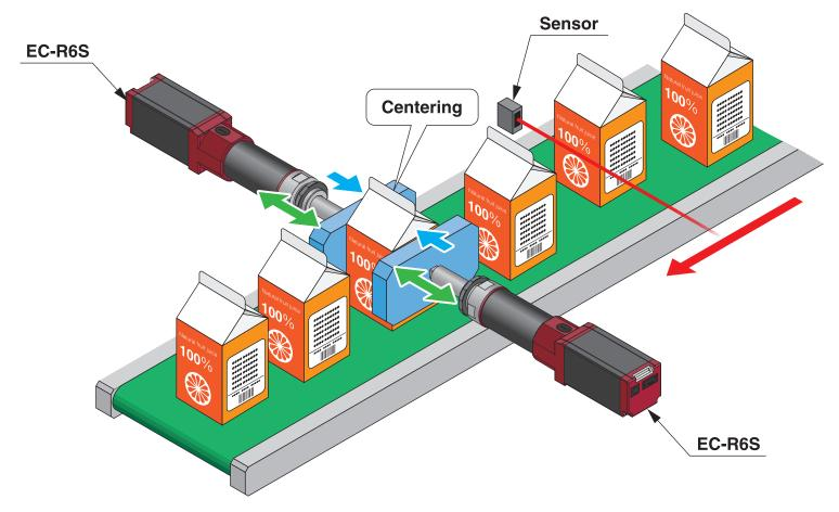
**Explanation** Previously, air cylinder was used in order to center the beverage packaging.
