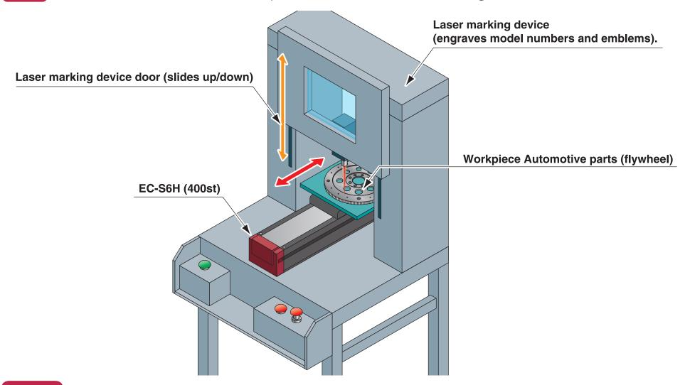
Explanation Conventionally, an air cylinder was used for this mechanism. However, there were difficulties in fine-tuning the transport speed and transport position. The Elecylinder is equipped with a feature that allows the product transfer position and A (acceleration), V (velocity), and D (deceleration) to be set using numerical input. This has reduced the time taken to adjust the position and the speed while ensuring a smooth operation.
