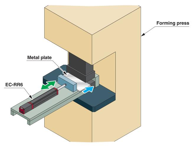
Explanation Conventionally, the metal plate was loaded manually by having a worker pushing it into the forming press.
