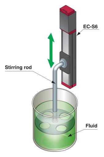
**Explanation** Initially, air cylinder was considered to be used for agitation, but decided to adopt the Elecylinder, which has a high degree of freedom in terms of amplitude and agitation speed.
