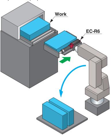
**Explanation** Conventionally, an air cylinder was used here, but it was motorized in order to remove the air piping.
